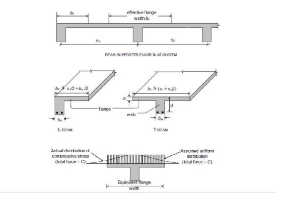
Figure. T-beams and L-beams in beam-supported floor slab systems
